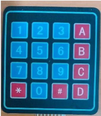
A blue matrix keyboard with a grid of buttons. The buttons are labeled with numbers 1-9, 0, *, #, and letters A, B, C, D.            | \$2,00  |
