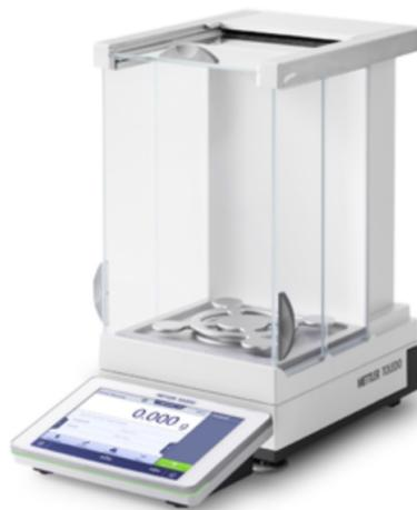
**Figura 3.21 Balanza XPR2003SC [43]**
