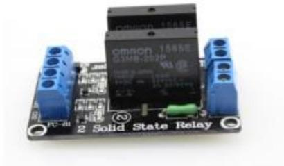
A two-channel relay module (HCMODU0115) featuring 2x Omron G3MB-202P solid state relays. A Solid State Relay is similar to a mechanic relay where it can be controlled through a digital signal. Solid State Relay generates no noise and has a much longer lifespan in compared to the traditional mechanic relay.
