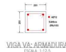
**VIGA VA: ARMADURA**
