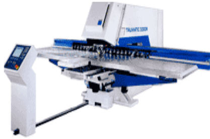
Figura 1.5 Press TRUMATIC 2020R FMC compact
