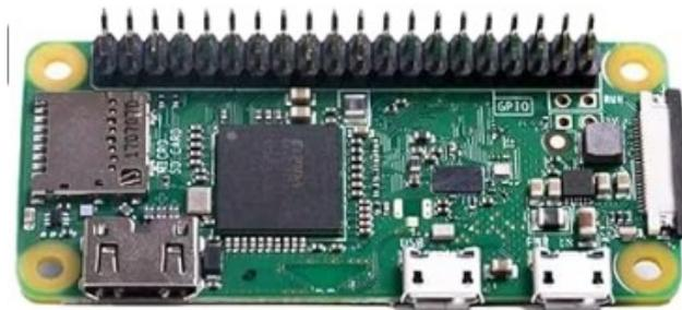
Figura 2.4: Raspberry Pi Zero
