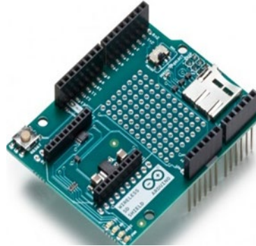
Figura 2.14 Módulo Arduino Wireless SD Shield [13]
