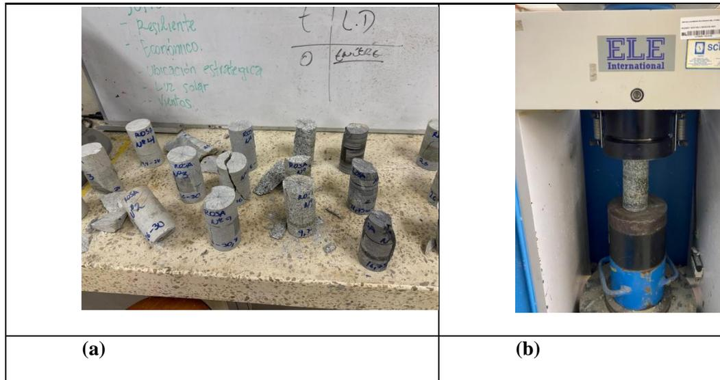
The maximum compressive strength is described as the stress required for the cylindrical core to generate a fracture in its structure. When conducting the test, the fracture will occur at the moment when there is a sudden drop in the applied load. The compressive force produced is in accordance with the ASTM D7012-04 standard [19], corresponds to:
