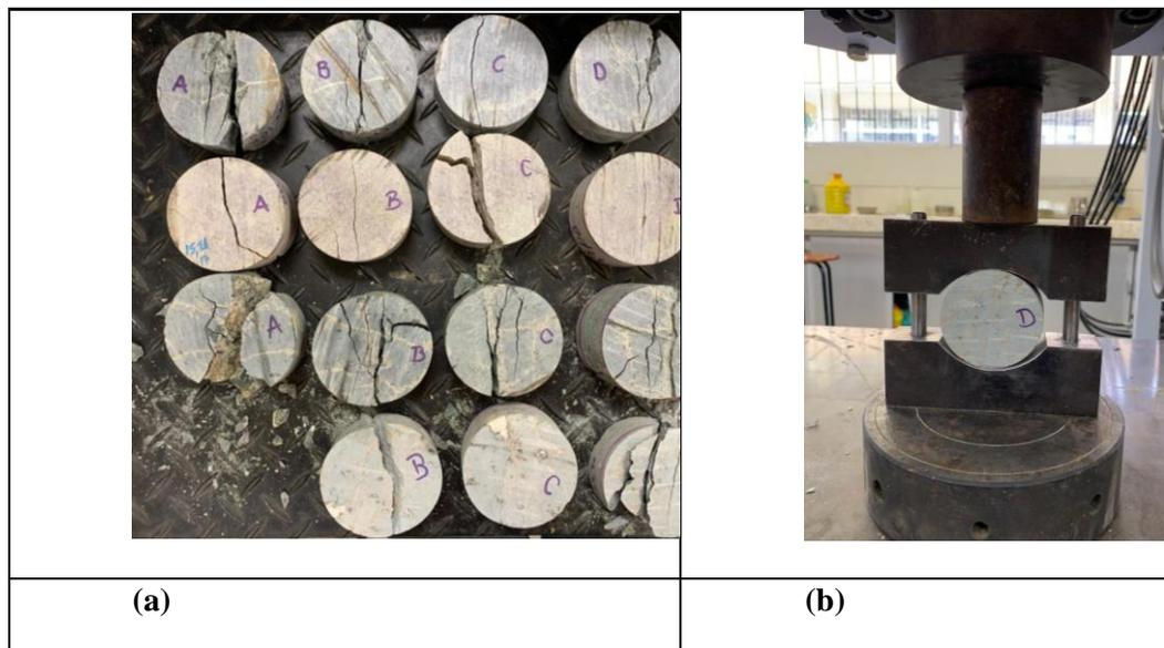
The test samples will be circular discs-cores with a thickness-to-diameter ( $t/D$ ) ratio between 0.2 and 0.75. The diameter of the sample must be at least 10 times greater than the largest mineral grain component. A diameter of 50 mm (NX) will generally meet this criterion (see figure 7). According to ASTM D3967 – 95 standard [20] The tensile strength of the specimen must be calculated as follows:
