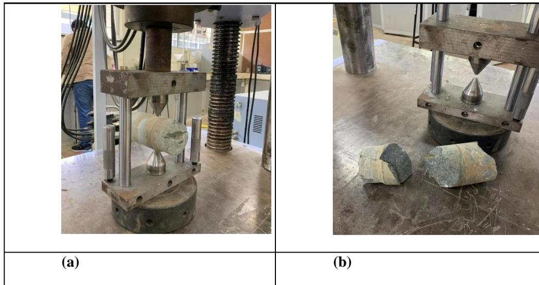
After recording the force applied by the piston on the rock sample to break it, the point load index is calculated using the following equation.
