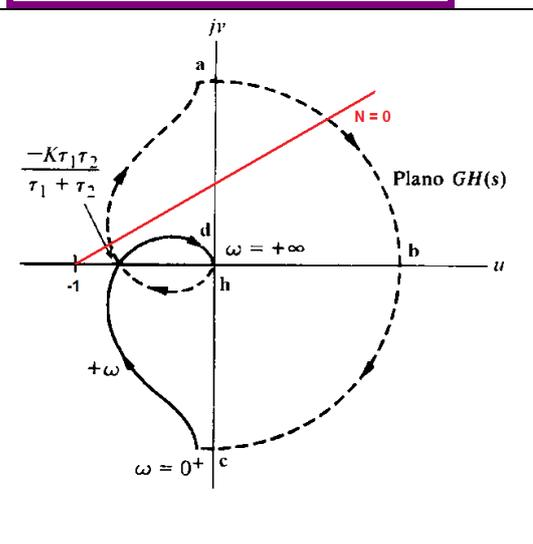
$$\text{Im}\{GH(\omega)\} = \frac{-K(1 - \omega^2 \tau_1 \tau_2)}{\omega(1 + \omega^2(\tau_1^2 + \tau_2^2) + \omega^4 \tau_1^2 \tau_2^2)} \Big|_{\omega=\omega_{cg}} = 0 ; \omega_{cg} = \frac{1}{\sqrt{\tau_1 \tau_2}} \rightarrow \omega_{cg} = 0.707$$
