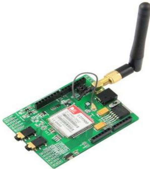
Figura 3.16 GSM SHIELD SIM900 [65]
