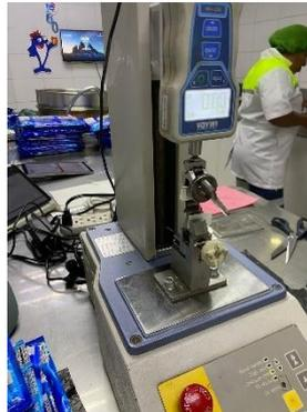
**Figura 2-9***Medición de resistencia de sello de funda verde*
