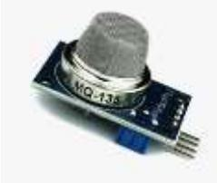
A photograph of an MQ-135 gas sensor module, which includes a sensor element and a small PCB with pins.                                                                    |
