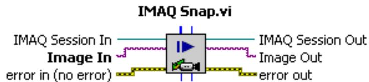
Acquires a single image into **Image out**. A snap is appropriate for low-speed or single-capture applications where ease of programming is essential.
