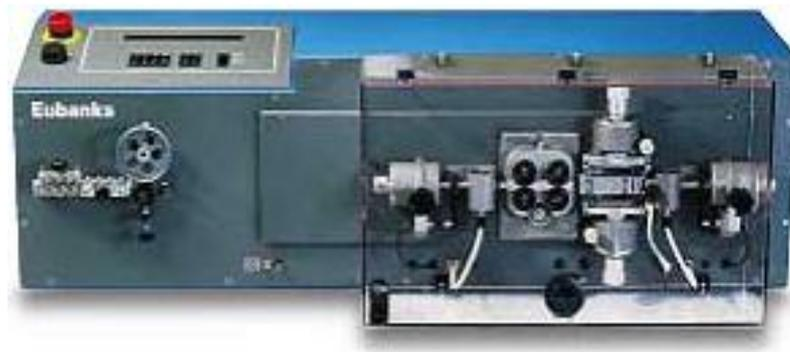
**FIGURA 2.12 MAQUINA CORTADORA EUBANKS**
