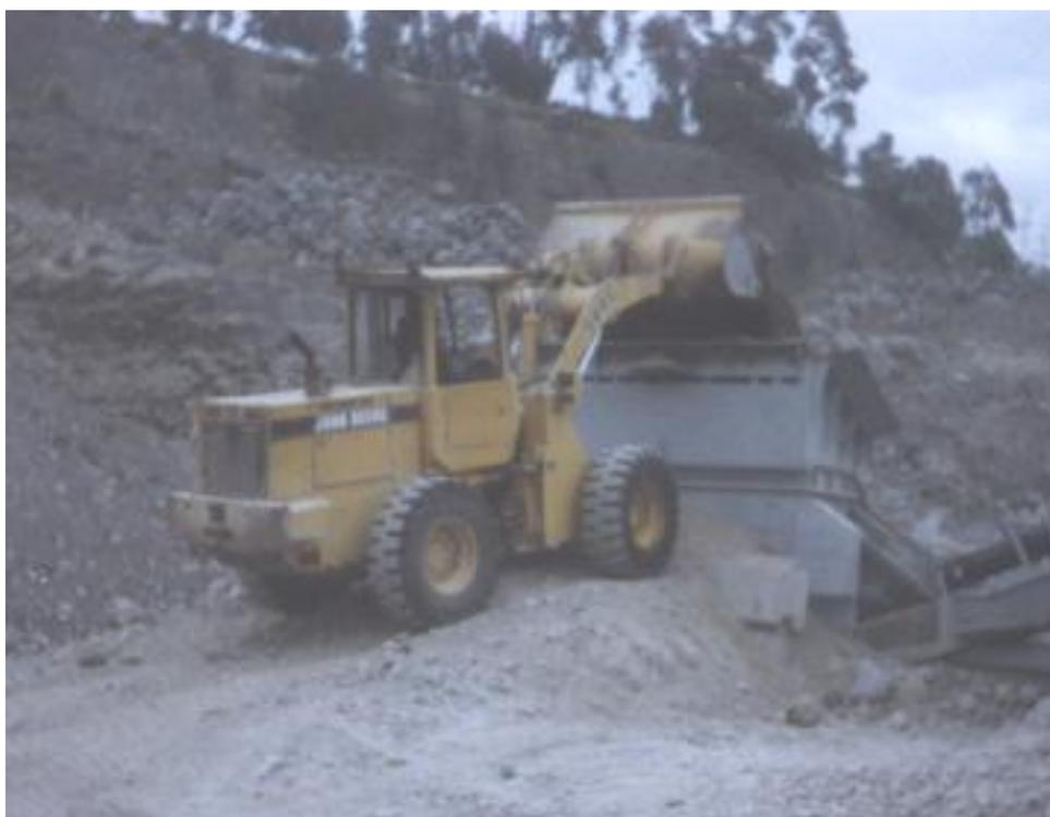
**FIGURA 1.3 TOLVA RECEPTORA DE MATERIAL**
