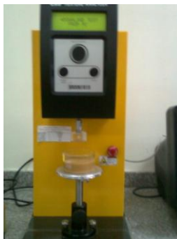
FIGURA 3.11 CT3- Texture Analyzer.
