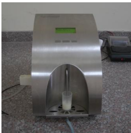
FIGURA 3.2 Lactoscan ó Milkanalyzer
