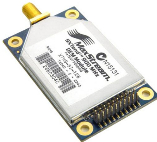
Fig. 2.3 Radio 9Xtend V. OEM 900 MHz MaxStream Digi
