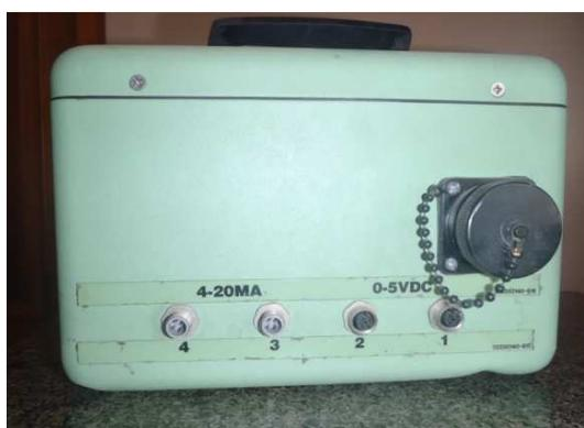
**FIG. 3.2 LOGAIR 2.0 DATALOGGER (4 CANALES)**
