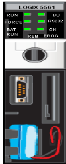
Panel frontal del ControlLogix
