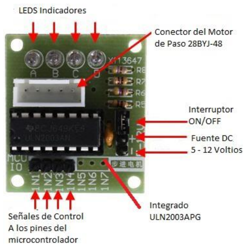
Fig. 6.18 ULN2003APG Driver
