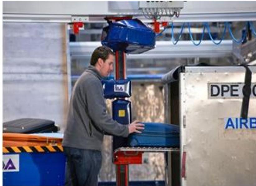
**FIGURA.90 SISTEMA ERGONÓMICO PARA CARGUÍO DE EQUIPAJES EN ULD**
