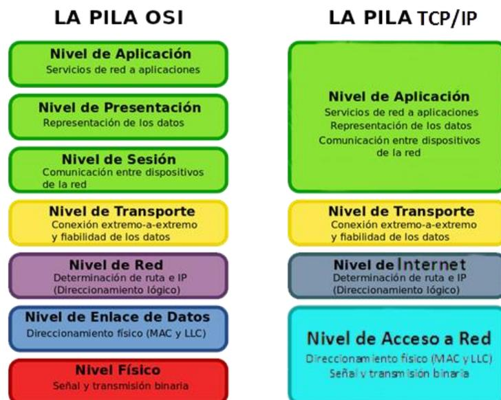
Figura 2.11 – Modelo TCP/IP [10]
