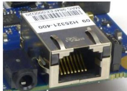
Figura 2.5 – Conector RJ-45 [5]
