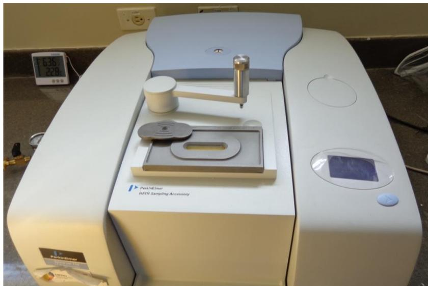
**FIGURA 3.5 ESPECTROSCOPIA INFRARROJA CON TRANSFORMADA DE FOURIER FTIR**
