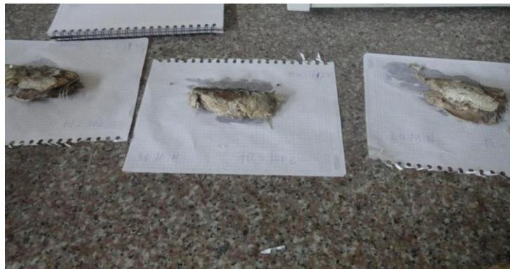
**FIGURA 2.8 MUESTRAS SACADAS A LOS TIEMPOS 20, 40 Y 60 MINUTOS TEMPARATURA 100°C.**
