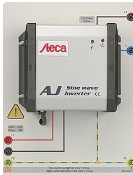
Figura 2.20 Inversor aislado 230V, (CO3208-1F). [1]
