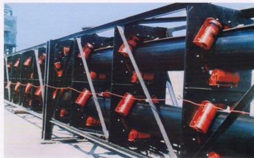
Fig. 3: Intermediate section of pipe conveyor
