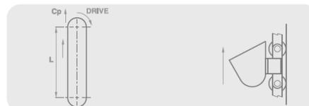
$$C_p = 9.81 [(w_b \times L) + (W_c \times L) + (L \times V_b \times \rho)] + D_f \text{ (N)}$$
