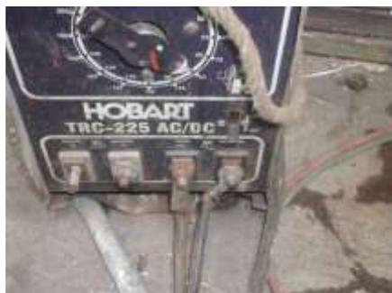
**FIGURA 2.18 MALAS CONEXIONES**
