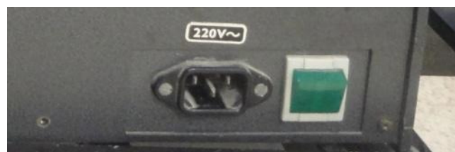
Figura 4.4: Conector 220V e interruptor principal del drive Terco MV4200.
