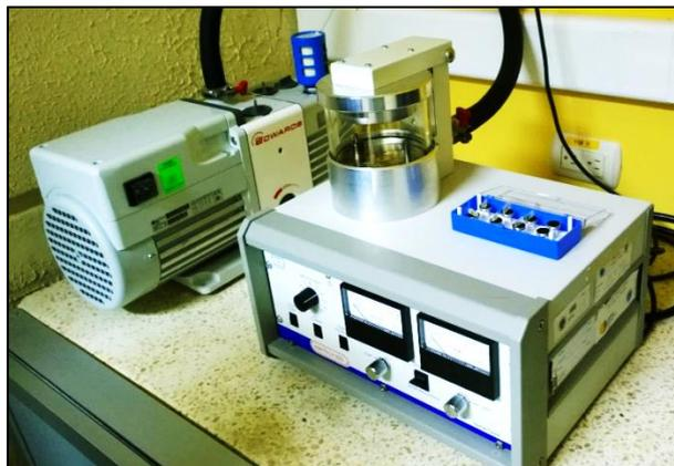
**FIGURA 3.59. RECUBRIDOR METÁLICO DE PLATINO**
