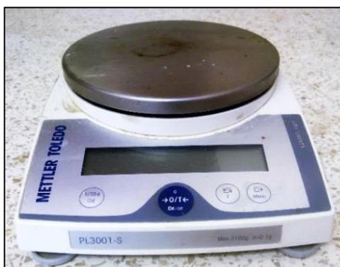
**FIGURA 3.51. BALANZA DIGITAL MAX 3100G-D 0.1G**
