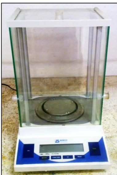
**FIGURA 3.50. BALANZA DIGITAL MAX 210G-D 0.001G**
