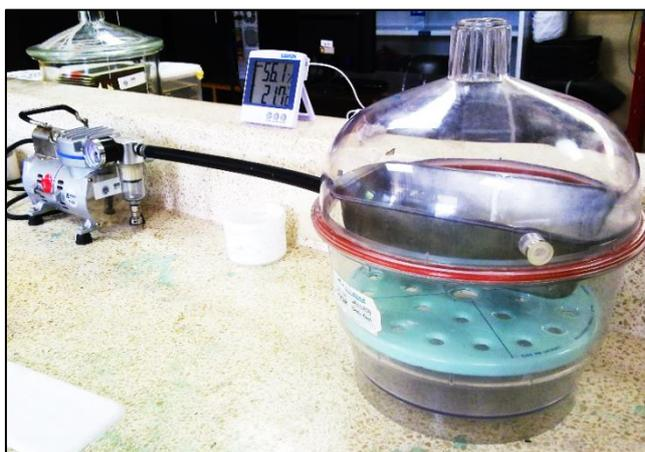
**FIGURA 3.52. CÁMARA DE VACÍO**
