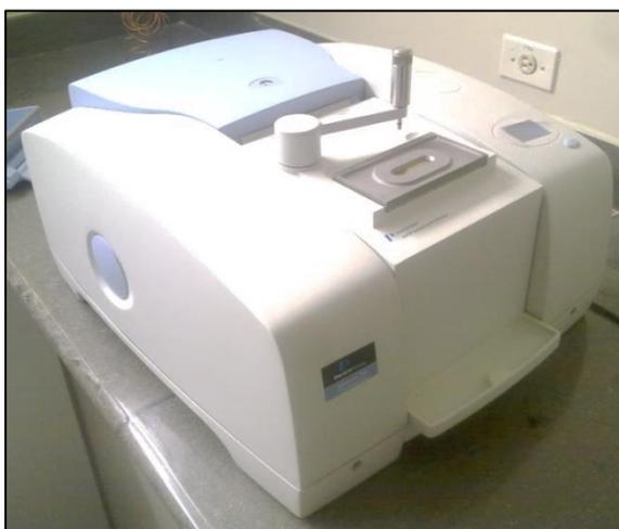
**FIGURA 3.55. ESPECTROFOTÓMETRO INFRARROJO POR TRANSFORMADA DE FOURIER (FTIR)**
