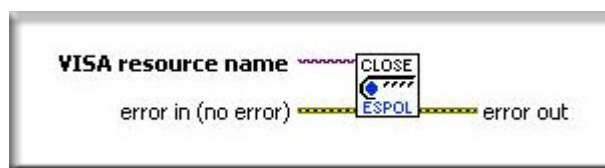
Figura 3.46 SubVI Espol Lab Conveyor Close
