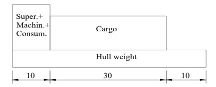
Weights on the ship are: hull: 250 tons, cargo: 600 tons, and, superstructure, machinery and consumables: 100 tons in the aft part of the ship; all weights may be assumed as uniformly distributed.
