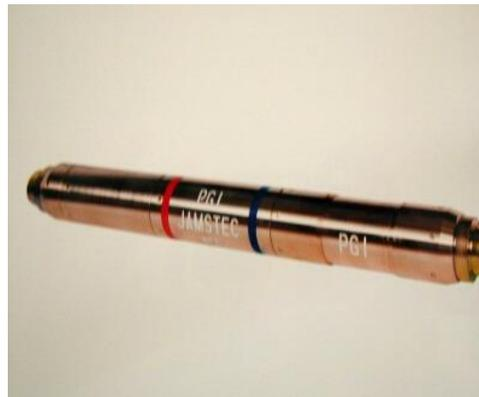
**Figura 3.4: Tsunami Sensor off Muroto Cape [30]**
