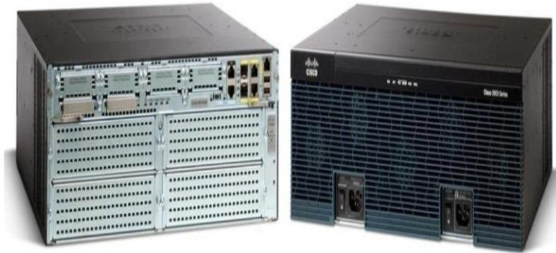
**Figura 3.19: Cisco 3900 Series Integrated Services Routers [37]**
