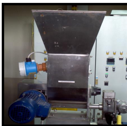
Figura 3.10: Sensor FTC-260 y tolva [18]
