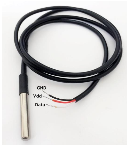
Figura 2.4: Sensor DS18B20 Waterproof [11]
