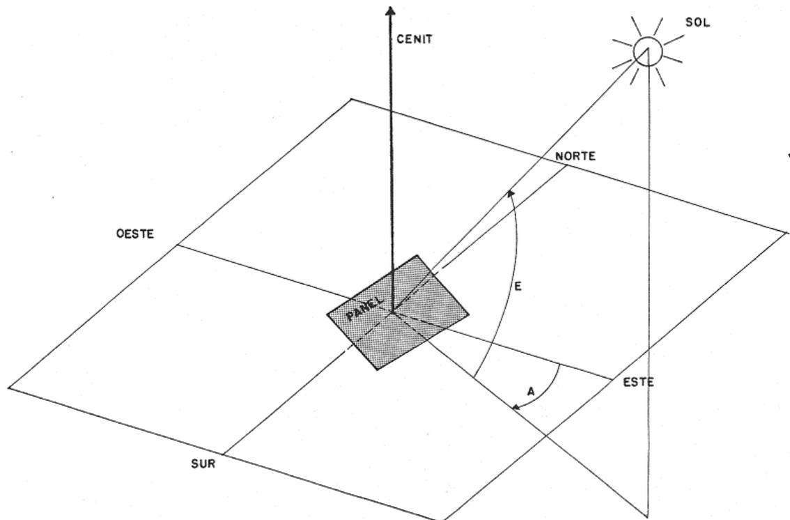
FIGURA 1.2 PANEL EN POSICION PERPENDICULAR AL SOL
