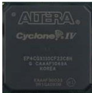
**Figura 2-2 FPGA Cyclone IV [4]**
