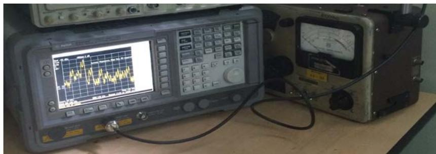
**Figura. 4. 1 Agilent E4404B SPECTRUM ANALIZER.**
