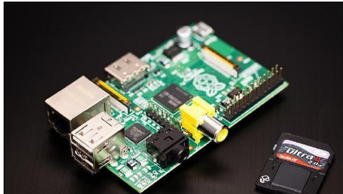
Figura 2.12 - Vista frontal placa Raspberry Pi b+ [12]
