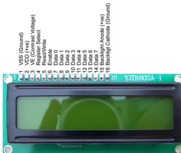
Figura 3.1 Pines del LCD 16x2 [ http://www.protostack.com/blog/2010/03/character-lcd-displays-part-1/ ]
