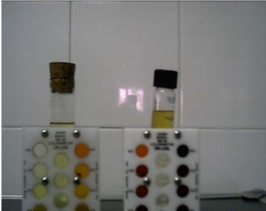
FIGURA A.8 COLORIMETRO CON COLORES ASTM
