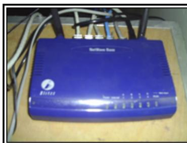
**Figura 2.1** Router - Switch Blitzz BWA-G11
