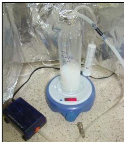
**Figura 3.7** Reactor batch
