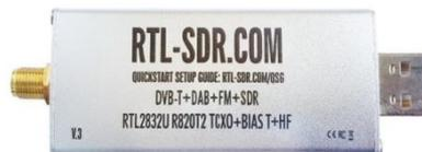
**Figura 2.4: RTL-SDR DVB-T, DAB, FM SDR [13].**
