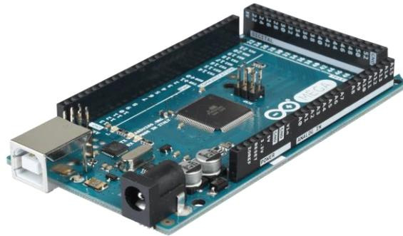
**Figura 2.5: Placa Arduino mega 2650**
