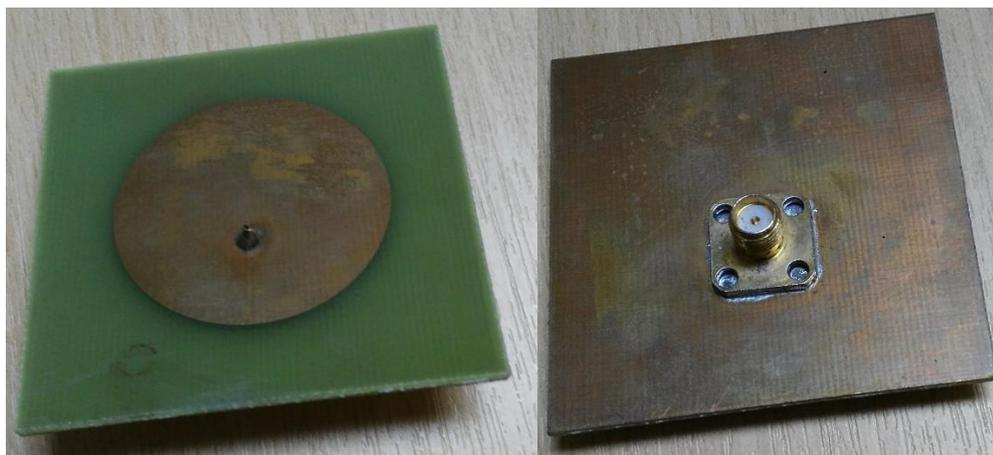
Figura 4.19 – Antena patch omnidireccional – circular
