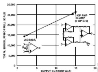
Figure 2. Three Op Amp IA Designs vs. AD620
