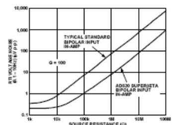
Figure 3. Total Voltage Noise vs. Source Resistance
