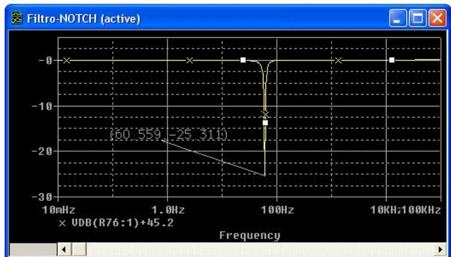
FIGURA 3.17 DISEÑO FILTRO NOTCH 60HZ
