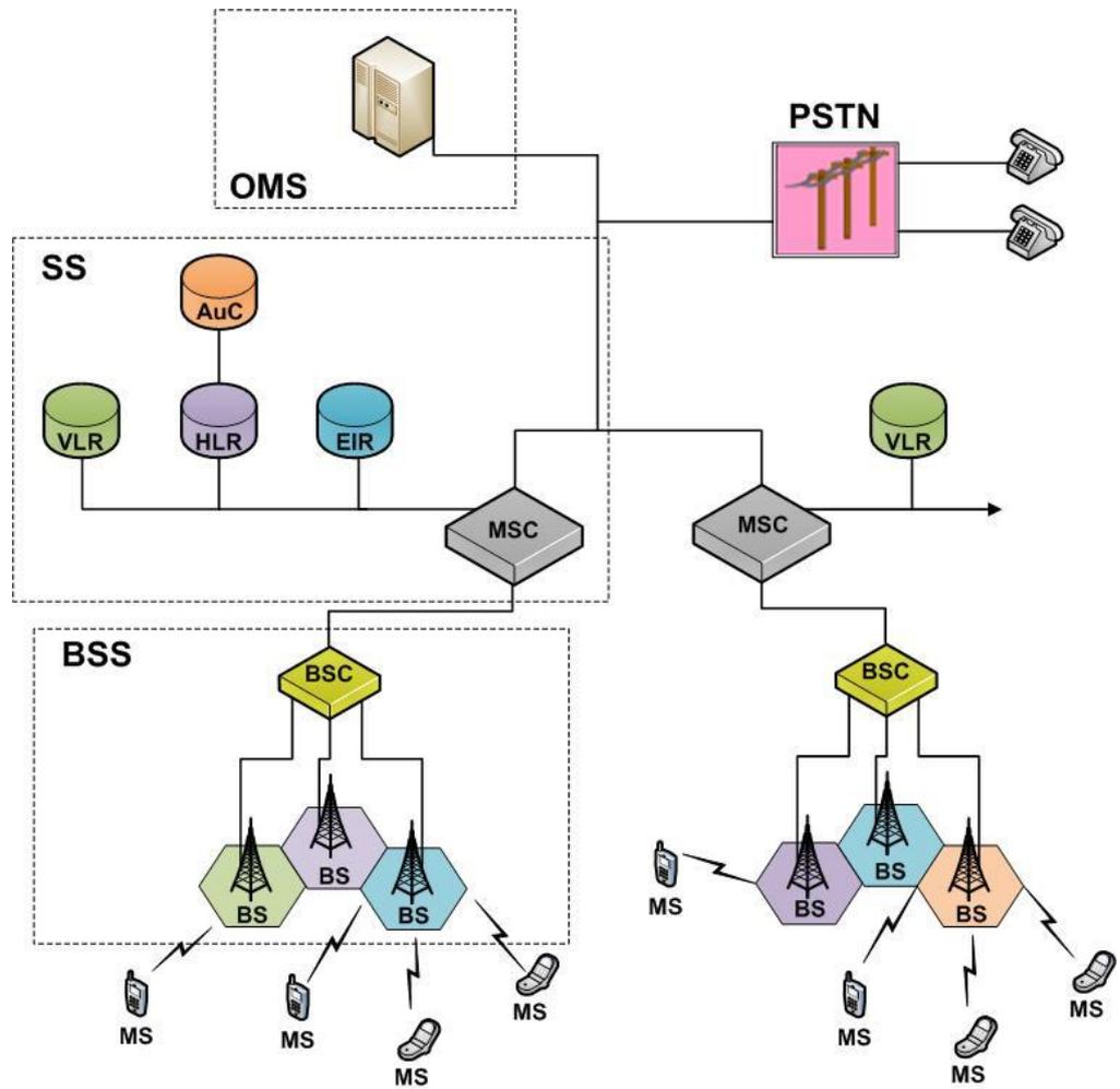
FIGURA 1.27 ESTRUCTURA DE LAS REDES CELULARES
