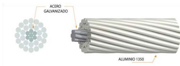
Figura 1.1 Conductor ACSR
