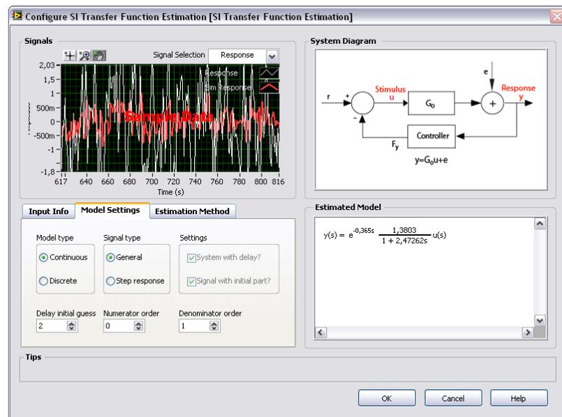
Figura 3.7: LabVIEW Asistente Conf. SI Transfer Function Estimation
