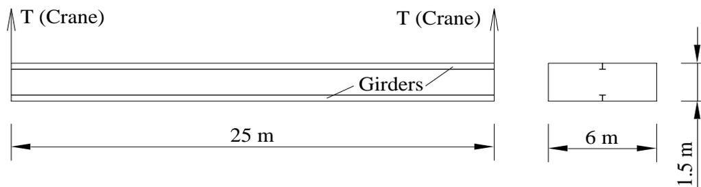
Bottom plate: 5 mm    Long.Girders:  $I_c$ : 1000cm<sup>4</sup>,  $A$ : 24cm<sup>2</sup>,  $d_m$ : 15cm (from web bottom)
